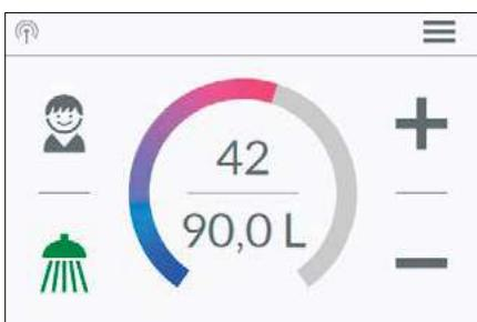
**Fill-Up:** Under "Fill-Up", tap on or to set the desired water quantity and then tap on "START" to activate Automatic mode. The view changes to the main control where the set quantity is displayed directly below the temperature display. Turning on the hot water tap starts the function and the set fill quantity counts down in litre increments according to the flow measurement.
