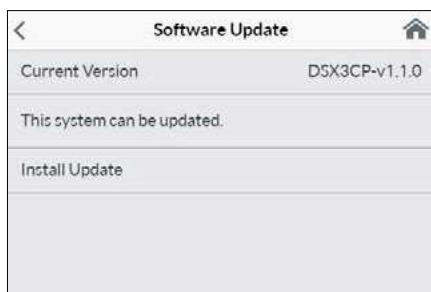
For an update the DSX Touch must be connected to a Wi-Fi network with internet access.
