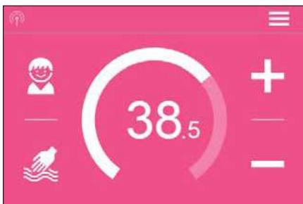
Eco active: The outlet temperature for all applications and the water flow are limited to an energy-efficient value. If the temperature is set higher via the temperature setting, the symbol starts to flash.
